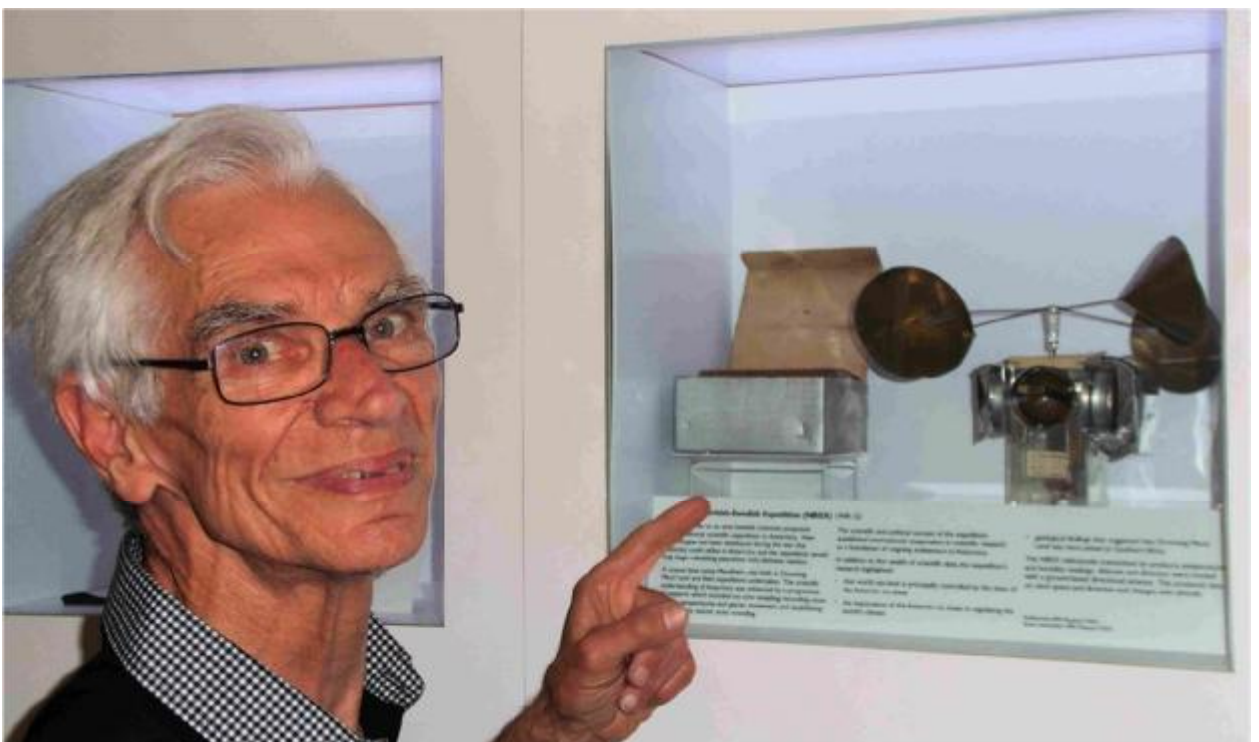
I couldn't resist a chuckle at this display, a sonde unit from the Maudheim expedition of 1949-52. It's mounted on its side! Someone saw the windmill part and assumed that to be an anemometer for wind speed. Of course, an ascending balloon moves together with the wind and so the apparent horizontal wind speed is always zero! That component should have the axis horizontal, so that it's turned by the air rushing past vertically as the whole thing ascends. This then turns a gear (a worm drive in ours, as I remember), and that turns a three-way switch to transmit the three readings (temperature, pressure and humidity) in succession for a few seconds each. I eagerly pointed it out to one of their guides.
